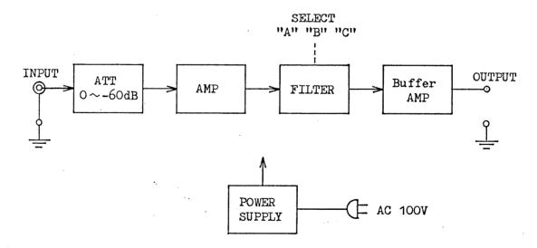
Note: Note that, since this instrument is an amplifier with aural compensation characteristics, it is possible that the amplifier is saturated with an excessively large input and the measurement becomes unsuccessful unless the output is monitored within the maximum output level by connecting an output meter to the OUTPUT terminal.
